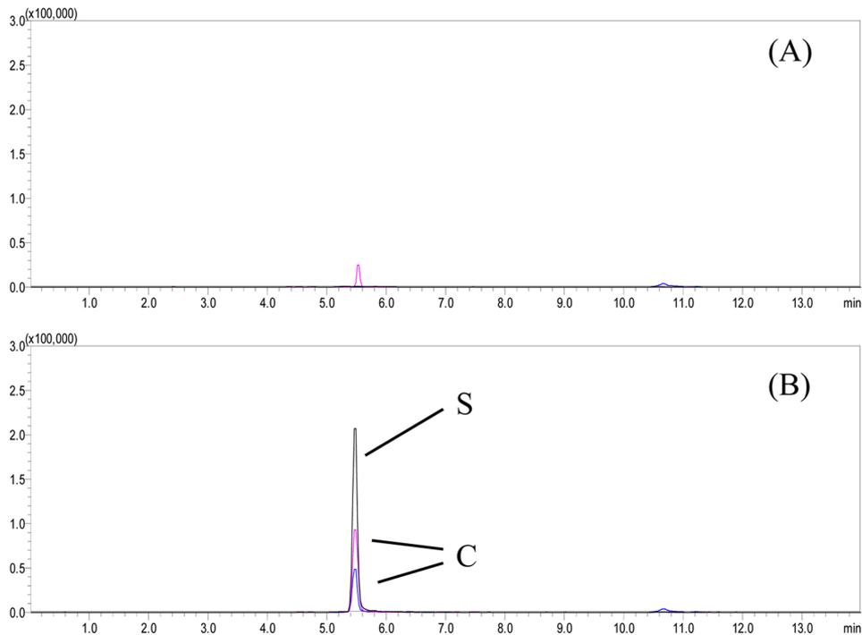
**Figure 3.** MRM chromatograms from blank halibut (A) and standard (5 ppb)-spiked halibut (B) analyses. S and C stand for the screening transition peak and the confirmatory transition peaks, respectively.
